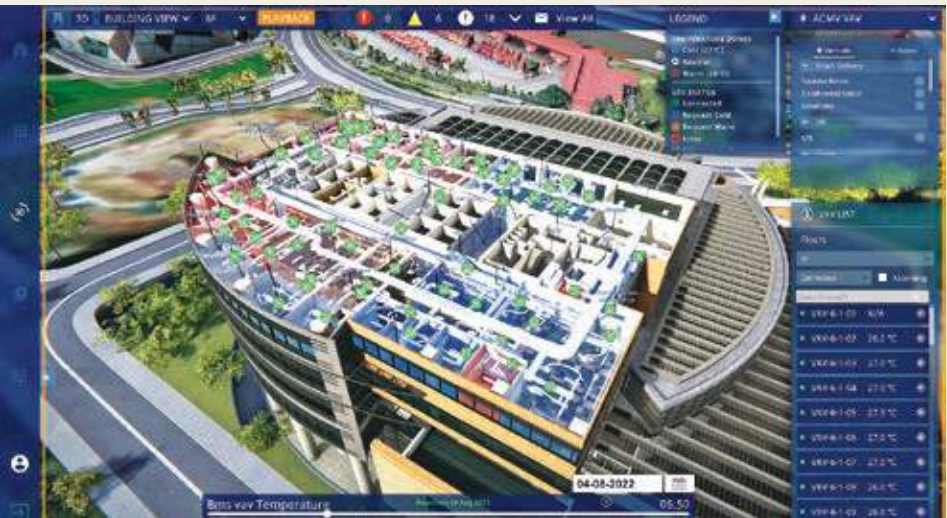
Cross-section of JTC Summit’s Digital Twin, showing almost real time data of the cooling system in the building Image courtesy of JTC
