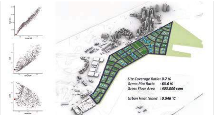
Generating various development options with procedural modelling and multi-objective optimisation to address urban heat impacts, developed in collaboration between the URA and SUTD Adaptive Design Lab Image courtesy of Cooling Singapore 2.0 project by the Singapore ETH Centre
